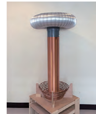
Tesla coil made by students
