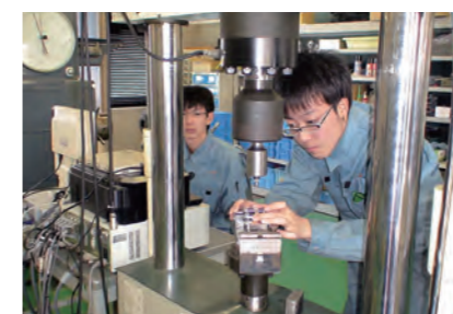
Fatigue Test of Metallic Materials
