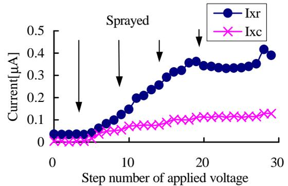
Figure 5. Change of dielectric property after the spraying of distilled water on HTV-SIR during the application of constant ac voltage. Conditions: Room temperature, amplitude of applied voltage is 50 Hz, 1,000 V (zero to peak). Averaging 100 times each point. Distilled water was sprayed on the HTV-SIR at the times shown in this figure.
