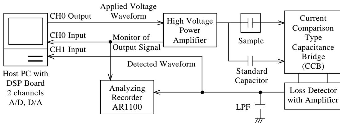
Figure 3. Schematic view of DSP measuring system.
