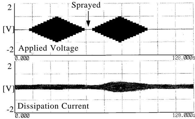
Figure 6. Applied voltage and unbalanced detected current waveform digitized by DSP system. Conditions: Room temperature, ac ramp voltage is applied two times sequentially. Maximum amplitude of applied voltage is 50 Hz, 1,000 V (zero to peak). Each step of applied voltage is constant during 100 cycles to carry out 100 times of averaging. Distilled water was sprayed on HTV-SIR before the second application of ac ramp voltage.
