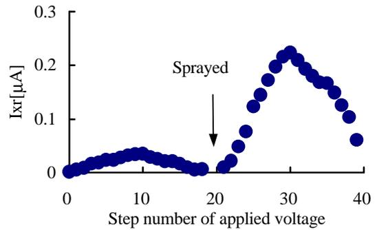
Figure 8. Change in dissipation current after the spraying of distilled water on HTV-SIR evaluated from Fig. 6.
