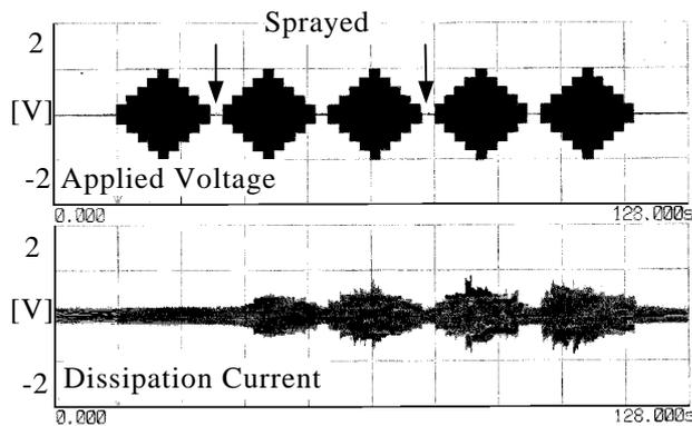
Figure 7. Applied voltage and unbalanced detected current waveform digitized by DSP system. Conditions are same as Fig.6 except the numbers of ac ramp voltages are 5 times.
