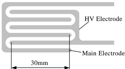
Figure 2. A pair of Interdigital Electrodes
