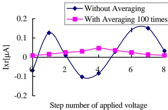
Figure 4. Evaluated result by DSP system of dissipation current with and without averaging of detected signals. Conditions: Room temperature, maximum applied voltage is 50 Hz, 1,000 V. All magnitudes of voltage and current are zero to peak values. Each voltage step is 200 V. Averaging is carried out 100 times for each step compared to capacitive component. Whereas, for
