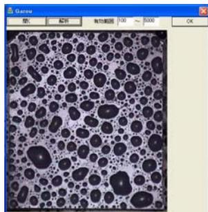
**Figure 2:** Interface of the developed image processing system. Menu buttons are Loading the image, Analyze the image, and lower and upper level of the size in pixels of the evaluated water droplets.
