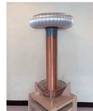
Tesla coil made by students
