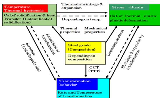
**Fig.1** Schematic view of the model of metallo-thermo-mechanics
