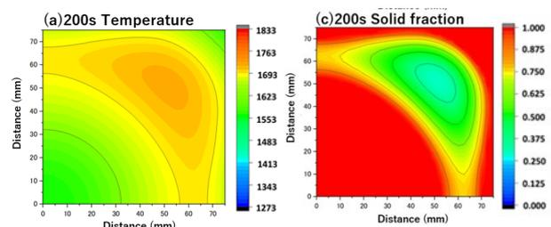
**Fig.2** Calculated distribution of temperature and solid fraction on 1/4 cross section of ingot at 200 s from teeming. (Insert casting, S50C, 150mmsquare Ingot, 60 $\Phi$ )
